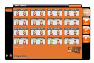
The master pointing device – touch pad of the notebook or conference pointing device – allows to select the mouse having the hand (green figurine) on a plan reproducing the arrangement of the class, with the names of the pupils.
