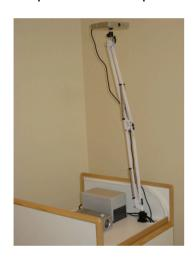
The infrared camera is mounted on an articulated arm over the cart so that the pen is always in the field of vision of the camera.
